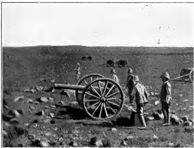
Artillery Firing with Smokeless Powder ; a fraction of a second after the discharge, as shown by the position of the men. The flash would have been shown if it had been possible to press the button on the instant. The smoke, if present, would have lingered long enough to have been caught by the camera.
